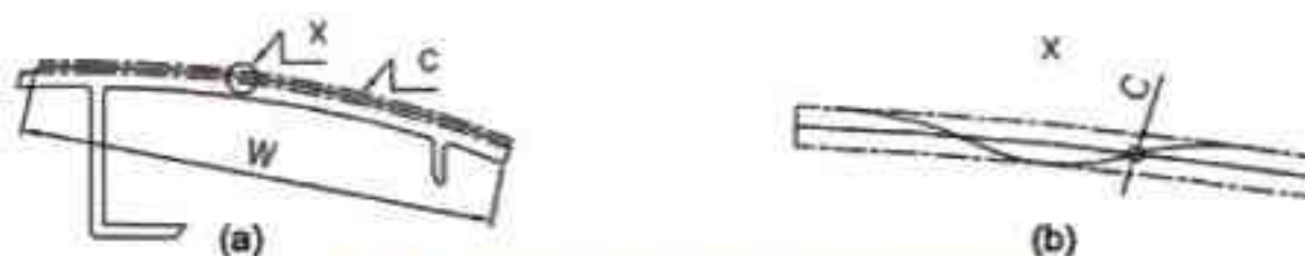
Fig. 7 – Definition of Contour Tolerances
